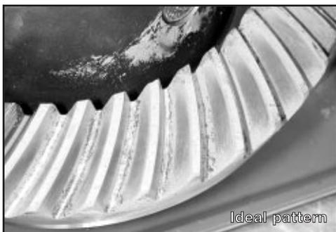
the teeth. If the contact pattern appears to be towards the heel or the toe of the ring gear teeth I pay no attention and **look only at the pattern position from face to flank**. The pattern will also change from heel to toe but in most cases an ideal heel to toe pattern can not be achieved. Trying to obtain a pattern that is centered from
