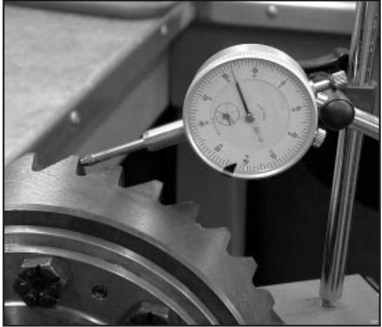
the pinion. If I want to increase the backlash by 0.007" I move the ring gear 0.010" farther away from the pinion. This is not exact for all ring & pinion sets, but it is a good general guideline.
