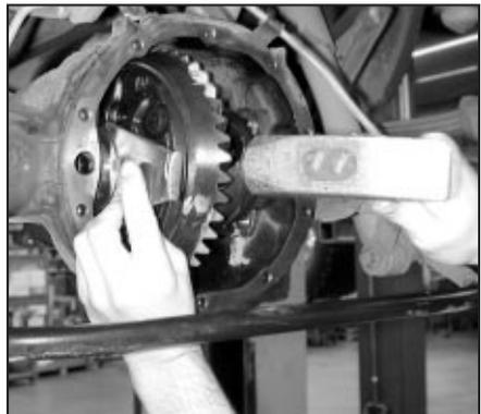
backlash with very little carrier bearing preload. After I have set the backlash I add shims to both the left and the right sides until I obtain the correct preload.
